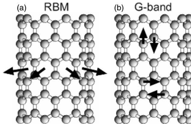
**Figure 3.** Schematic picture showing the atomic vibrations for (a) the RBM and (b) the G band modes.
