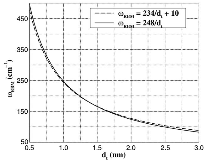
**Figure 4.** RBM frequencies  $\omega_{\text{RBM}} = A/d_t + B$  versus nanotube diameter for: (i)  $A = 234 \text{ cm}^{-1} \text{ nm}$  and  $B = 10 \text{ cm}^{-1}$ , for SWNT bundles [16] (dashed curve); (ii)  $A = 248 \text{ cm}^{-1} \text{ nm}$  and  $B = 0$ , for isolated SWNTs [3, 17] (solid curve).
