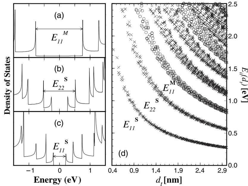
**Figure 2.** DOS for a (a) armchair (10, 10) SWNT, (b) chiral (11, 9) SWNT and (c) zigzag (22, 0) SWNT obtained with the tight binding model from [13]. (d) Shows the electronic transition energies  $E_{ii}$  for all the  $(n, m)$  SWNTs with diameters from 0.4 and 3.0 nm using a simple first-neighbour tight binding model [14]. Distortion from this simple one-electron model is expected for the lower energy transitions  $E_{11}^S$  and for SWNTs with  $d_t < 1$  nm.
