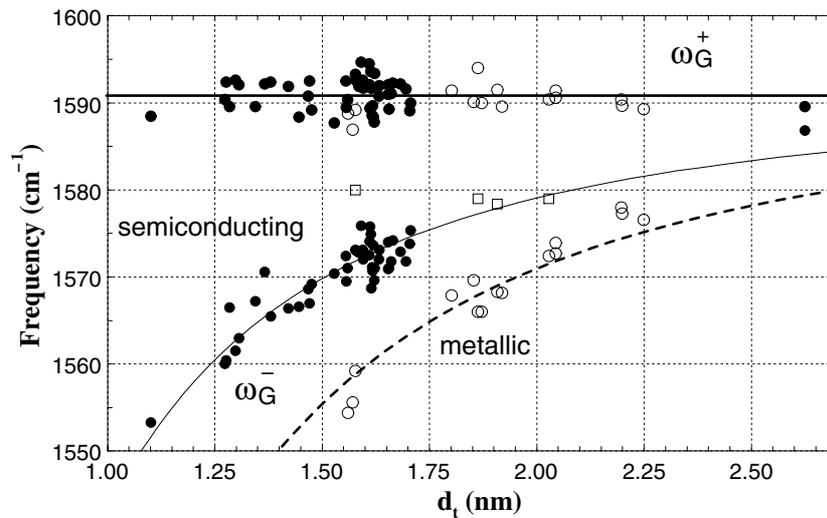
**Figure 7.** Diameter dependence for  $\omega_{G^+}$  and  $\omega_{G^-}$  for several isolated semiconducting and metallic SWNTs. Filled and open symbols apply for semiconducting and metallic tubes, respectively. The lines are fit to the experimental points (see table 1).
