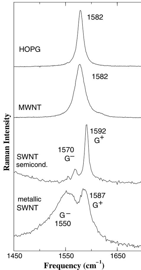
**Figure 6.** G band for highly ordered pyrolytic graphite (HOPG), MWNT bundles, one isolated semiconducting SWNT and one isolated metallic SWNT. The multi-peak G-band feature is not clear for MWNTs due to the large tube diameters (see section 10).
