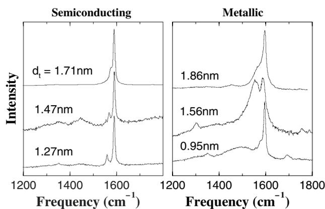
**Figure 9.** Raman signal from three isolated semiconducting and three isolated metallic SWNTs showing the G and D band profiles. SWNTs in good resonance (strong signal with low signal to noise ratio) show practically no D band. Spectra in bad resonance shows noisy background with a peak at  $\sim 1450 \text{ cm}^{-1}$  (e.g., see second trace for semiconducting SWNTs).
