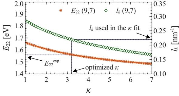
FIG. 1. (Color online) Left and right vertical axes show, respectively, the  $E_{22}$  and  $l_k$  dependences on  $\kappa$  for a (9,7) SWNT. The plot shows how the optimized  $\kappa$  is obtained for a given SWNT in a HiPco sample (data from Ref. 7).
