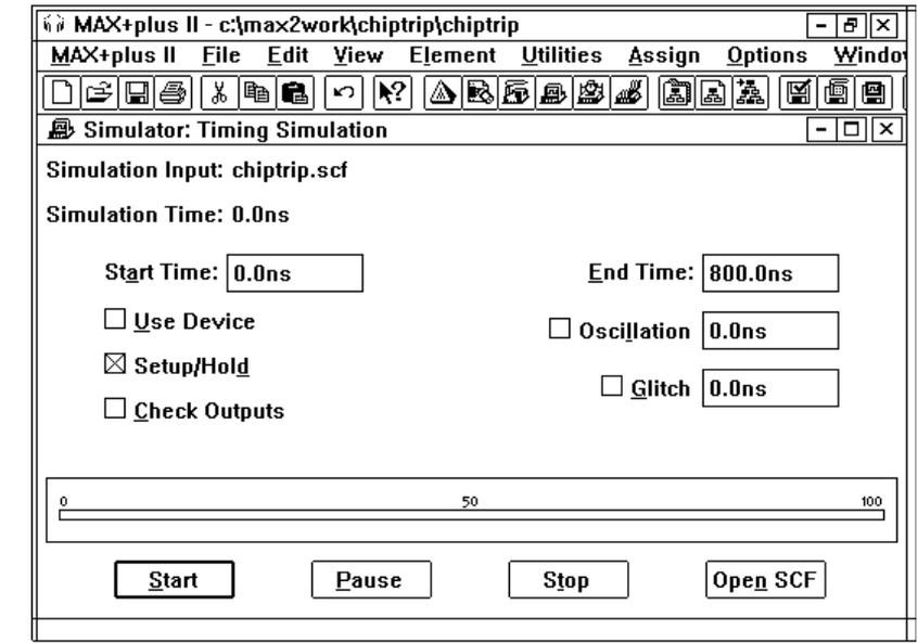
The designer either defines input stimuli with a straightforward vector input language or draws waveforms directly with the MAX+PLUS II Waveform Editor. Simulation results can be viewed in the Waveform Editor or Text Editor and printed as waveform or text files.
