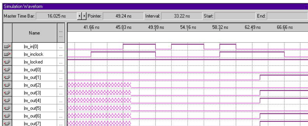
Figure 25. Bit Mapping Sample Waveform
