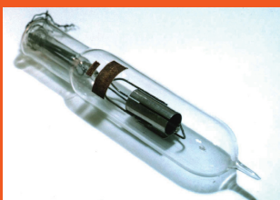
*Prototype of The divided anode-type magnetron when invented
