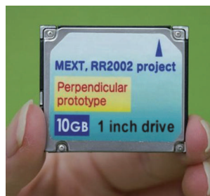
△ Prototype of 1 inch size HDD (10GB)
