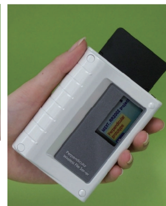
△ Prototype of 1 inch size HDD (10GB)
